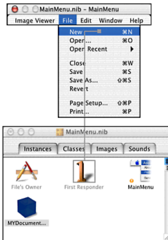
Figure 9.10. A connection line from the File, New menu item to the First Responder icon is shown with the target outlet and the newDocument: action selected.
