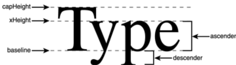
Figure 11.2. Fonts are measured by their total point size as well as ascender, descender, xHeight, and capHeight dimensions.
